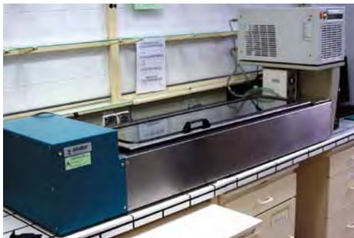
Figure 2.27. General view of the elastic recovery test set (photo by ORLEN Asphalt sp. z o.o., courtesy of ORLEN Laboratorium sp. z o.o.)
