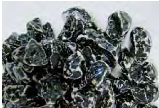
Figure 2.33. Aggregate samples after the test (method A) as per PN-EN 12697-11 (photo by ORLEN Asphalt sp. z o.o.)
