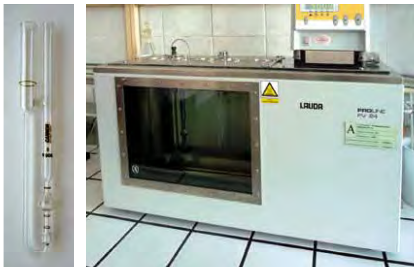
Figure 2.16. General view of the BS/IP/RF capillary viscometer and apparatus used for kinematic viscosity testing (photo by ORLEN Asphalt sp. z o.o., courtesy of ORLEN Laboratorium sp. z o.o.)
