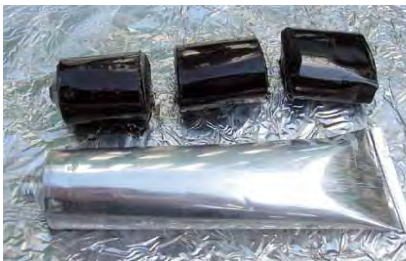
Figure 2.31. General view of the filled and sealed tube for the “tube test” and of the modified bitumen sample cut into three sections (photo by ORLEN Asphalt sp. z o.o., courtesy of ORLEN Laboratorium sp. z o.o.)
