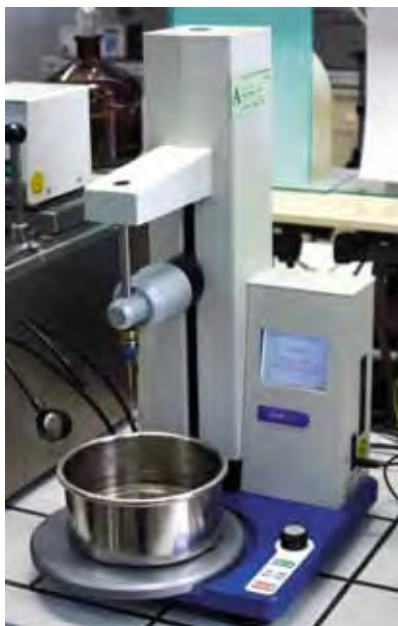
Figure 2.2. General view of the penetration test equipment with a bitumen sample (photo by ORLEN Asphalt sp. z o.o., courtesy of ORLEN Laboratorium sp. z o.o.)
