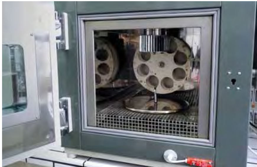
Figure 2.24. General view of the RTFOT short-term ageing test set (photo by ORLEN Asphalt sp. z o.o., courtesy of ORLEN Laboratorium sp. z o.o.)
