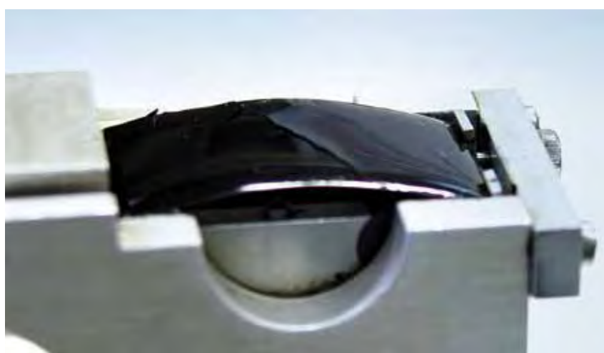
Figure 2.9. View of a bitumen sample on the plate placed on the semi-automatic set after the test – a bitumen layer crack can be seen (photo by ORLEN Asphalt sp. z o.o., courtesy of ORLEN Laboratorium sp. z o.o.)
