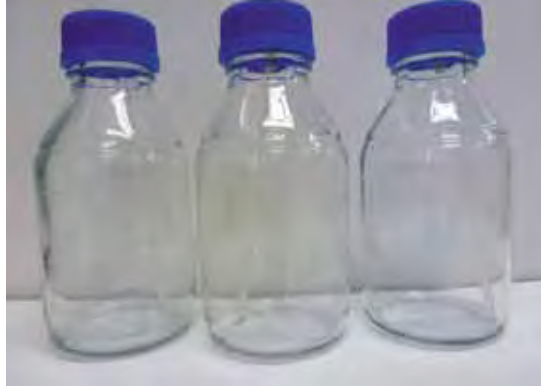
Figure 2.32. Bottles for testing binder elutriation from aggregate (method A) on the rolling machine acc. to PN-EN 12697-11 (photo by ORLEN Asphalt sp. z o.o.)
